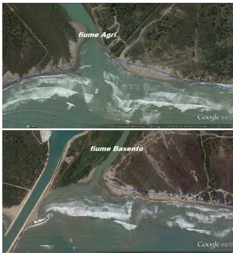
Fig. 5 - Coastal erosion near the mouths of the Agri and Basento rivers following the storms of late 2013.
