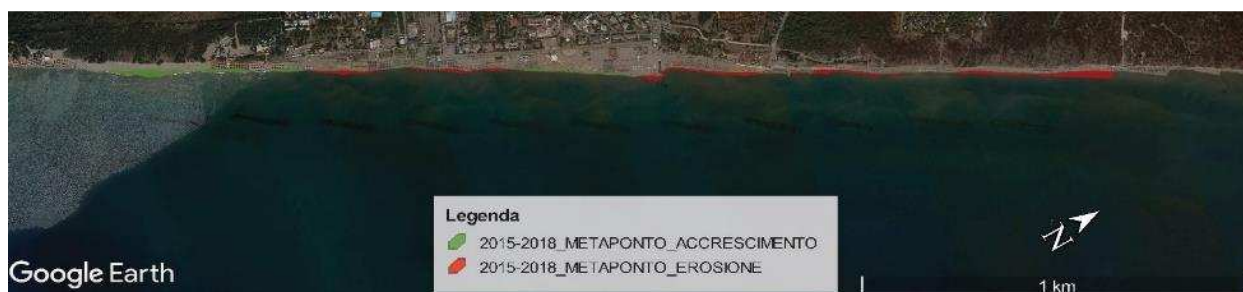
Fig. 6 - Submerged barrier to protect a stretch of Ionian Basilicata coast: comparison between 2015 2018 coastline.
